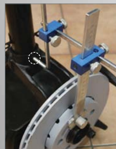
Unscrew the fixing bolt from the disc and mount the wheel alignment tool on the opposite hub wheel
