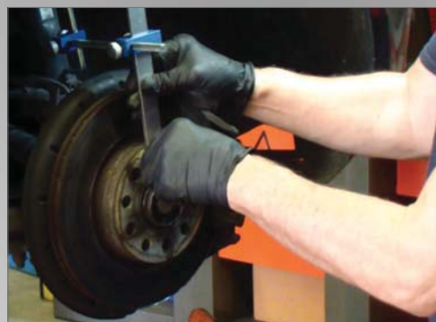
Adjust the pointing measuring tool against the fixing shock-absorber seat
