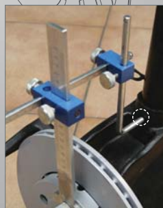
Adjust the pointing measuring tool against the fixing shock-absorber seat
